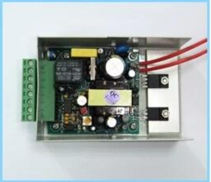
The switch power supply with 12v 3a output dc 110V-240V AC input and used with access control system.
