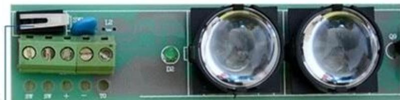
Tamper switch, when the invaders destroyed or disassembled, tamper switch will trigger the alarm immediately bounce.
