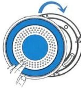
Align the siren with the base, rotate by clockwise
