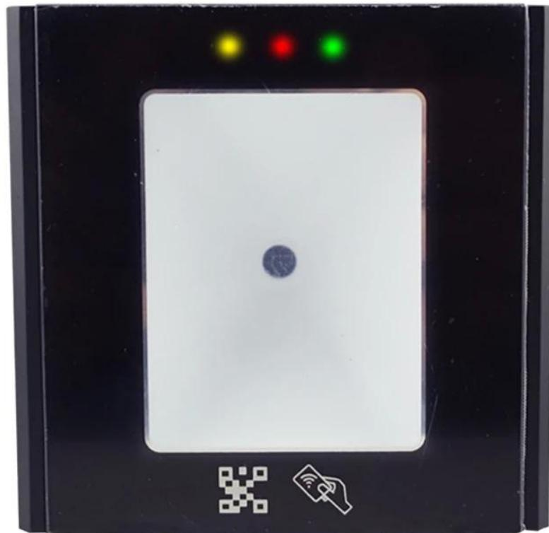
**1. Access control QR and RFID Reader with WG output**
