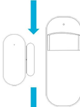
When a Door/Window Sensor detects a door/window opening, the sensor sends a signal to the panel letting the hub know there has been an intrusion.
