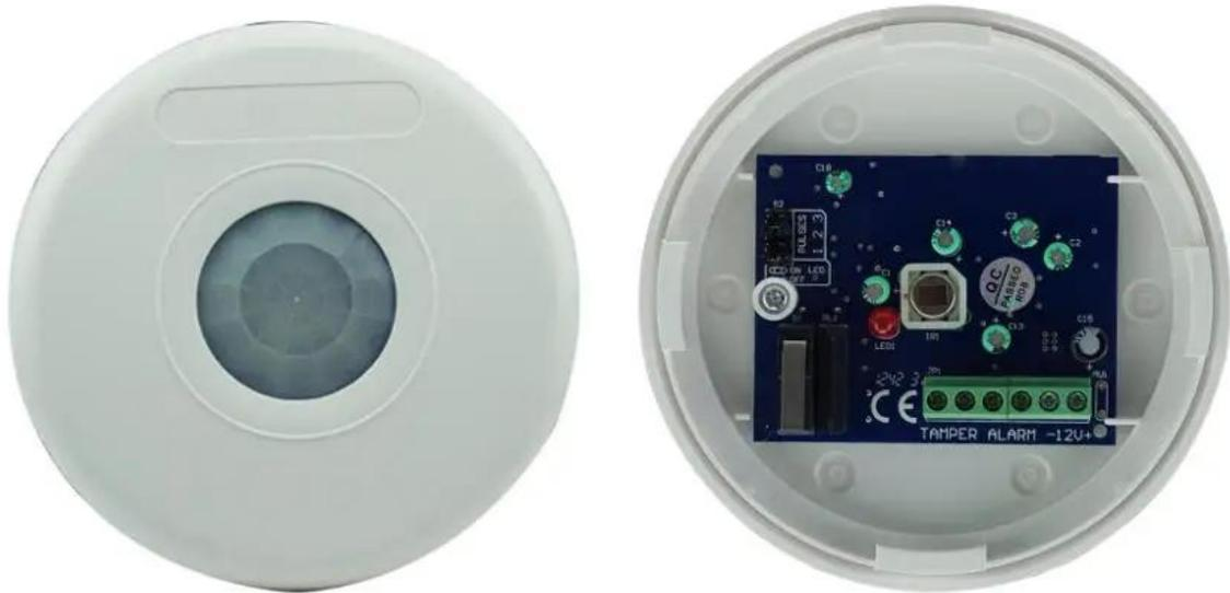
1.Ceiling Mounted Infrared Motion Sensor
