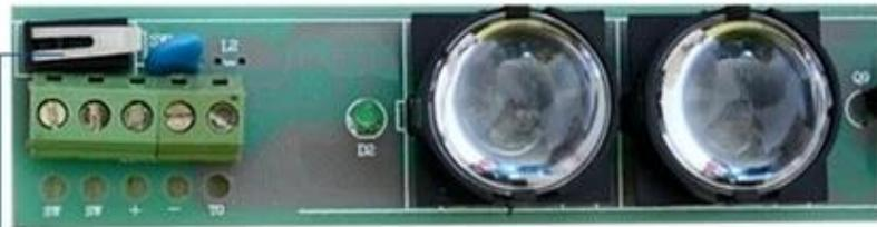
Tamper switch, when the invaders destroyed or disassembled, tamper switch will trigger the alarm immediately bounce.
