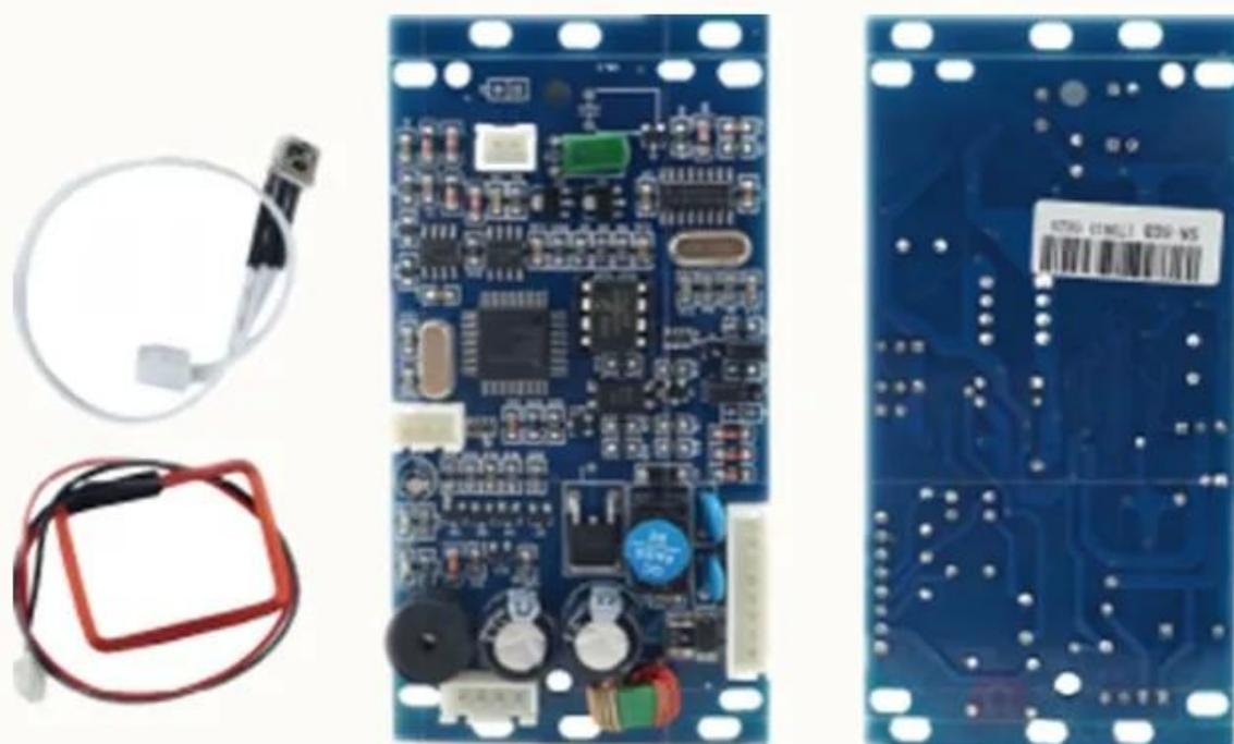
**Access control embedded standalone reader EM 125KHz**
