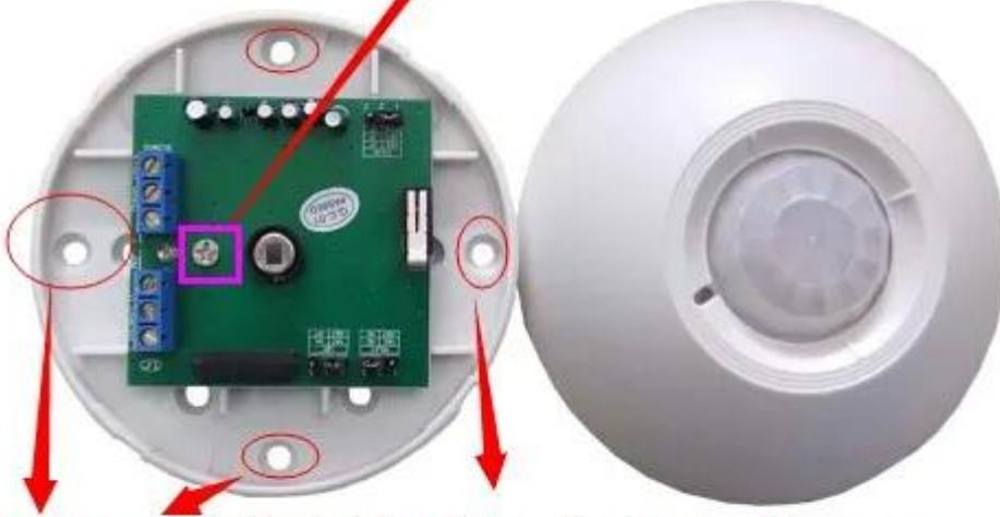
the red round is the hole to set the detector on ceiling , you also can take out the PCB and build again after setting on the ceiling.
