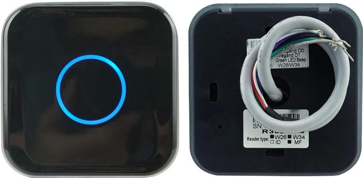
1. Waterproof door access control IC Card reader with WG26/34 adjustable
