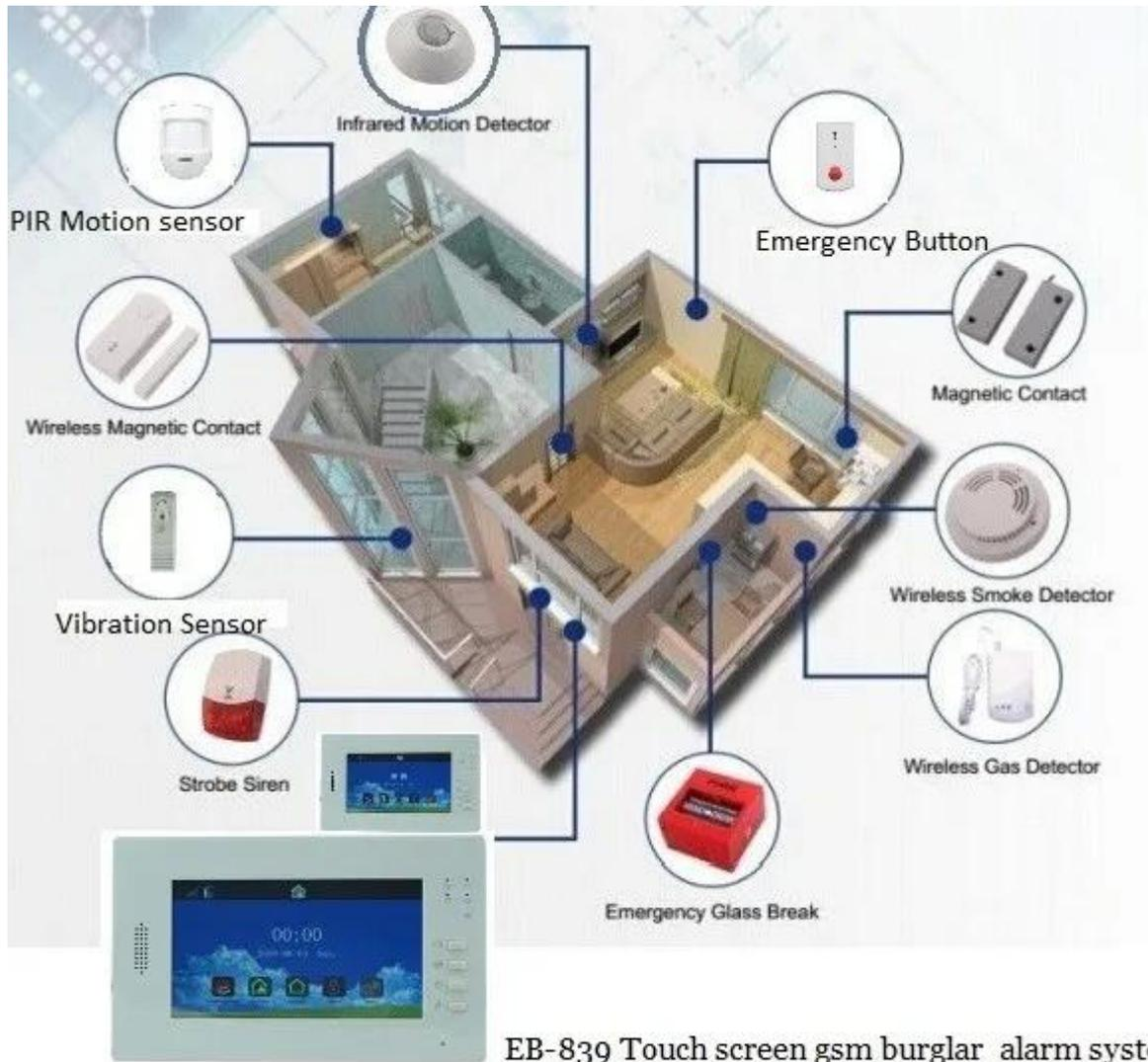
EB-839 Touch screen gsm burglar alarm system with CID monitoring dial
