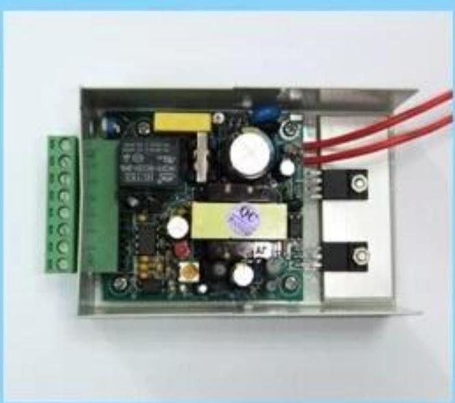
**The switch power supply with 12v 3a output dc 110V-240V AC input and used with access control system.**
