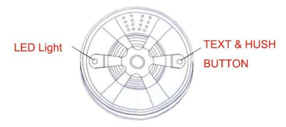
The detector adopts the reflection principle of smoke particles that can reflect infrared light The main circuit includes a MCU processing Section, an infrared-emitting portion and an infrared receiving portion.
