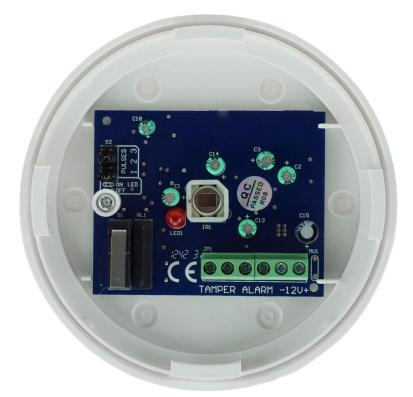
Pulses jumperLED indicatorLED jumperPIR sensorTamper deviceWire port
