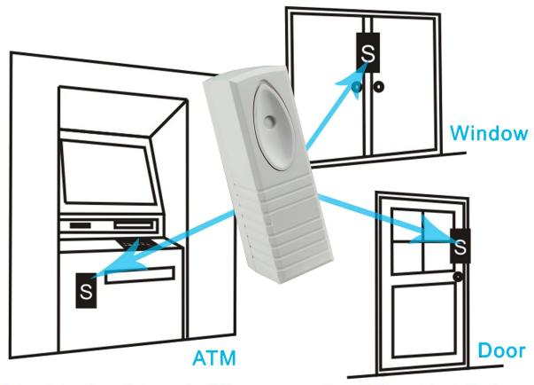
Note: detecting distance is different according different installation environment:concrete 1.5m , brick wall 2.5m, iron and steel 3m, glass 3.5m, wood 3.5m
