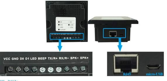
VCC: DC12+; GND: DC12-; D0:DATA0; D1:DATA1; LED:light control; BEEP:beep control ; TX/R+:RS232+/RS485+; RX/R-:RS232-/RS485-; SPK-、SPK+: Temporary undefined; RJ45: It can be used to connect network and use PC software to set parameters of reader card; it is suitable for HTTP mode communication; micro-USB:Suitable for USB virtual keyboard and USB virtual serial communication mode;
