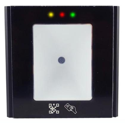
1.Access control QR and RFID Reader with WG output
