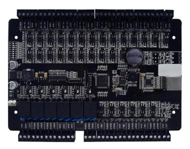
Suitable for all kinds of WG format door access control system WG26/34(adjustable)
