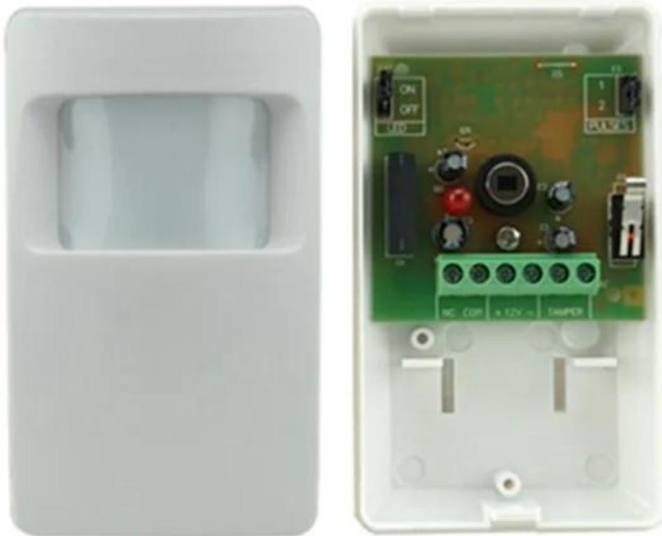
1.Wired Infrared PIR Motion Sensor
