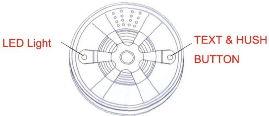
The detector adopts the reflection principle of smoke particles that can reflect infrared light. The main circuit includes a MCU processing Section, an infrared-emitting portion and an infrared receiving portion.
