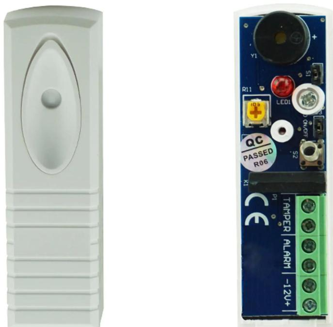
1. Wired ultrasonic vibrate motion detector
