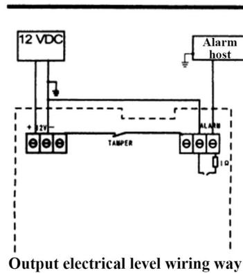
Output electrical level wiring way
