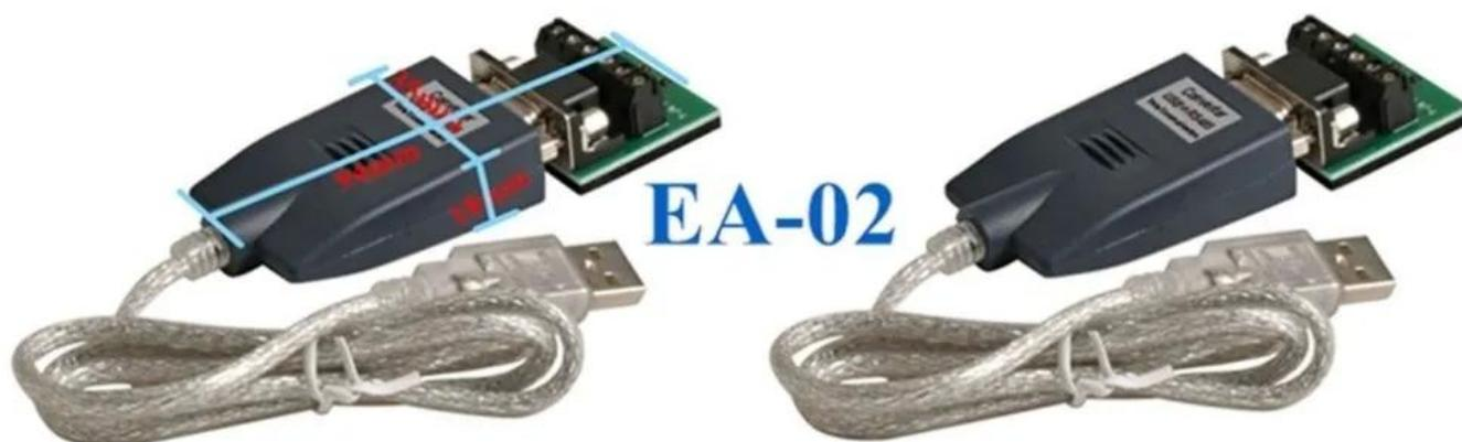
**1.Converter USB to RS485 interface compatible with EIA/TIA RS-232, RS-485 standard**
